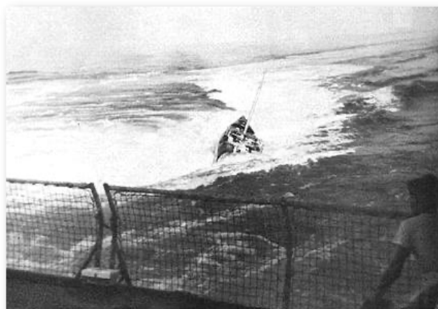
The USSR boat wallows in the sea, suffering damage to her bow, sail, and forward decking.
